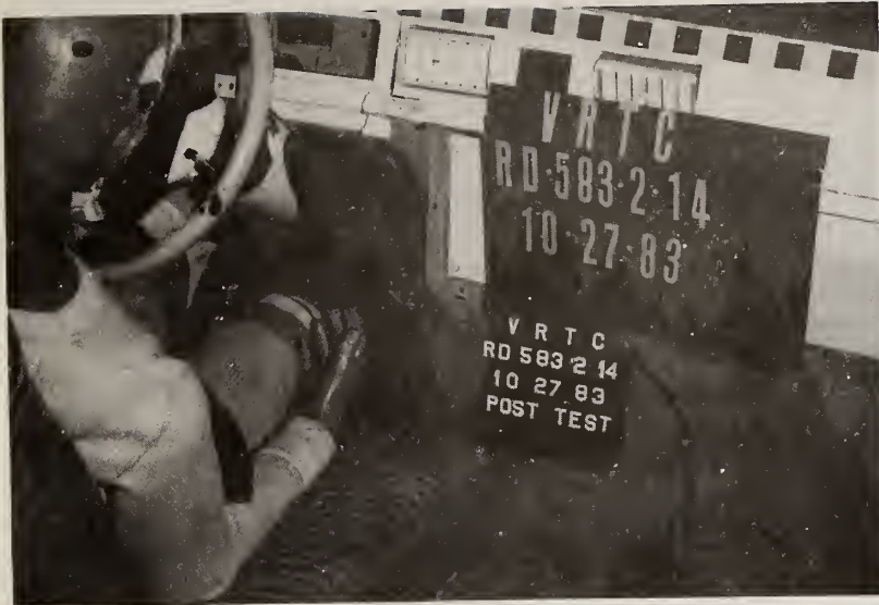
Right Knee Impact Area, Test 14 (No Contact)
